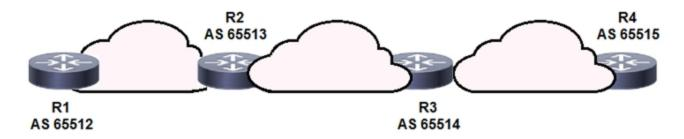
Refer to the exhibit. BGPsec is implemented on R1, R2, R3, and R4. BGP peering is established between neighboring autonomous systems.
